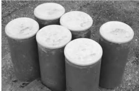
Figure 4.4-4 Sealed concrete cylinders cast at site for lab testing.
