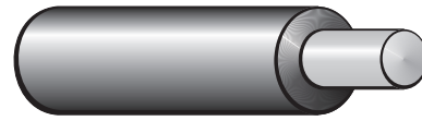
First, strip the wire to expose the correct amount of wire for the termination you’ve selected.
