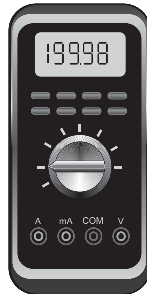
A modern multimeter can measure amps, ohms and volts.
