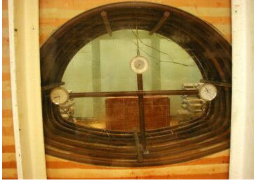
Figure 5: Detail of the tunnel with reinforcement and measuring equipments. and
