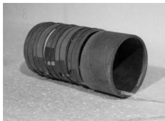
Figure 2: Equivalent of the tunnel lining with inner diameter of 76 mm created by hardened paper used in the model experiment.
