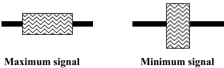
FIGURE 9.13 The proper device location.
