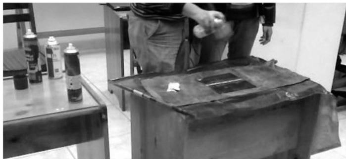
FIGURE 9.37 Using spray for developer, penetrate, and cleaner.
