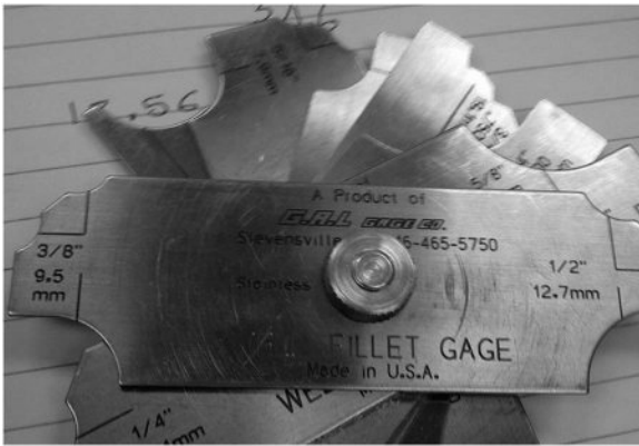
FIGURE 8.17 Fillet weld thickness test.
