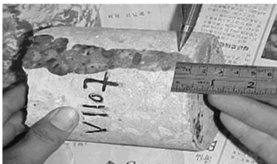
FIGURE 9.14 Carbonation depth measurement.
