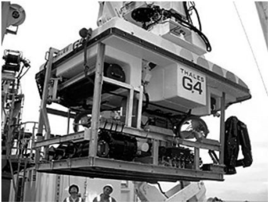
FIGURE 9.44 ROV subsea inspection.
