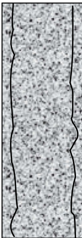
FIGURE 8.9 Cracks due to corrosion or concrete covered not enough.
