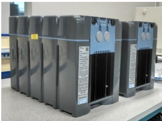
Figure 2.13. Soft Li-ion batteries: nominal voltage 48 V, charge current 32 A, discharge current 44 A, energy 3,900 Wh, specific energy 130 Wh/kg, 4,300 cycles at a discharge depth of 80% (L2EP HEI Lille)
