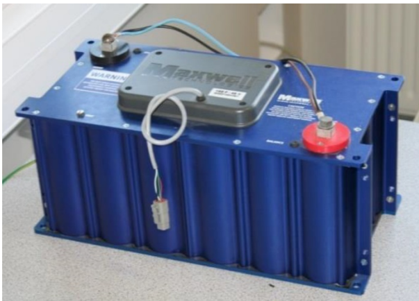
Figure 2.17. MAXWELL supercapacitor: voltage of 48 V and capacity of 165 Farads (L2EP HEI Lille)
