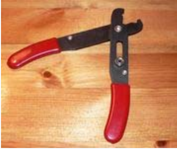
A simple manual wire stripper
