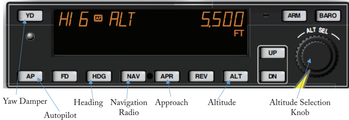
Figure 1.6: Interface panel for a simple autopilot.
