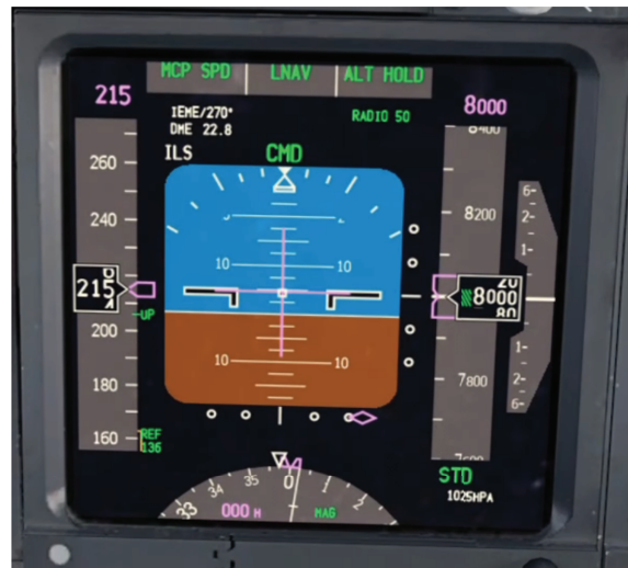
Figure 4.3: Primary flight display of a Boeing 737 MAX 8.
