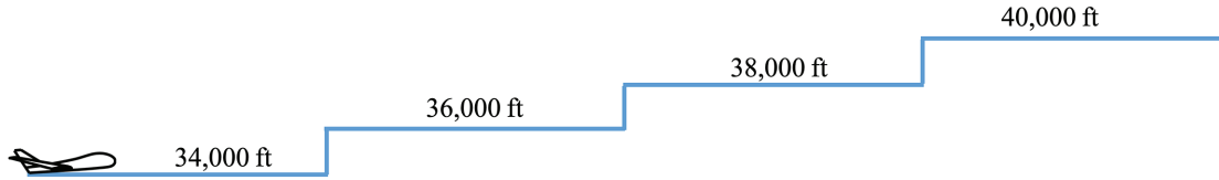
Figure 4.20: A typical step-climb.
