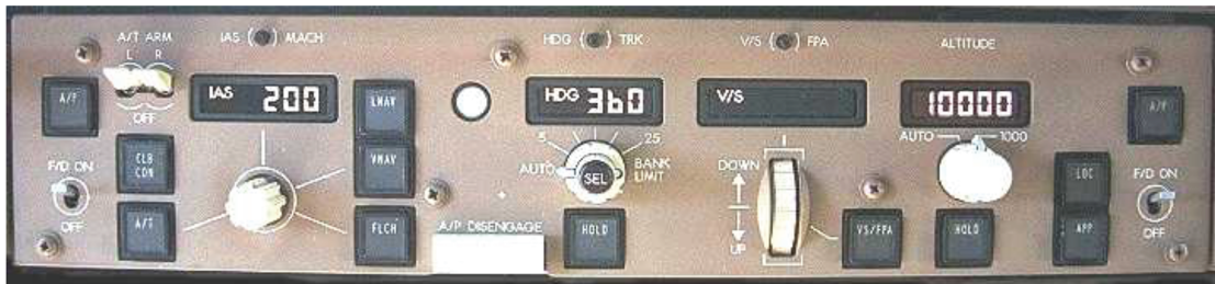
Figure 1.7: Boeing 777 mode control panel.
