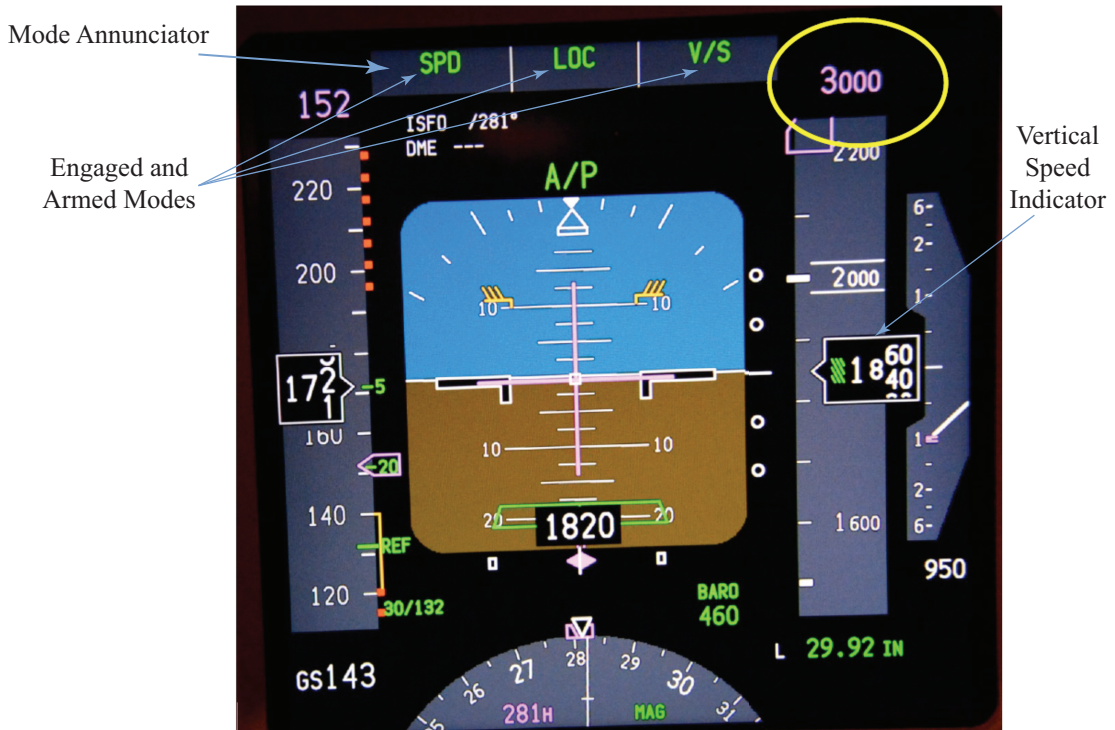
Figure 1.8: Primary flight display of a Boeing 777.
