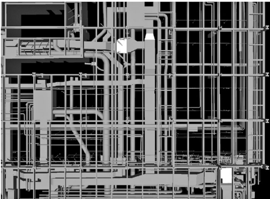
Figure 5.6.4 Scanned area of actual existing systems—modeled from a point cloud (area scanned with a laser scanner). (Image courtesy of Turner Construction, Sacramento, California.)
