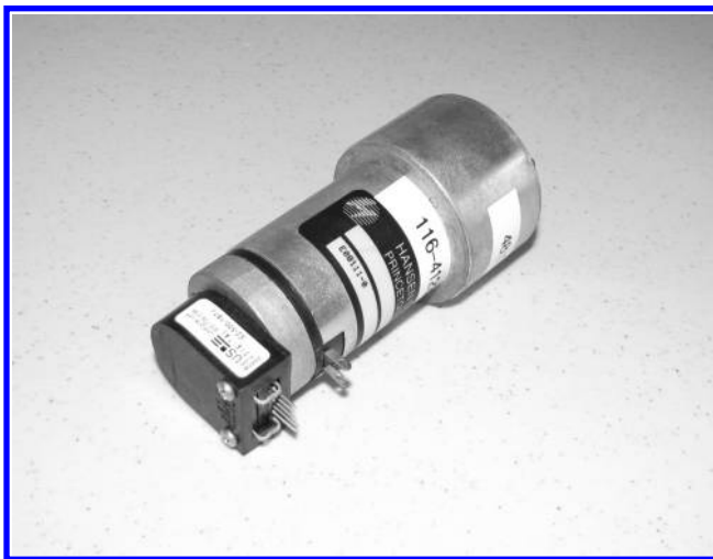
FIGURE 8.5 Motor/encoder combination as delivered by Hansen Corp.
