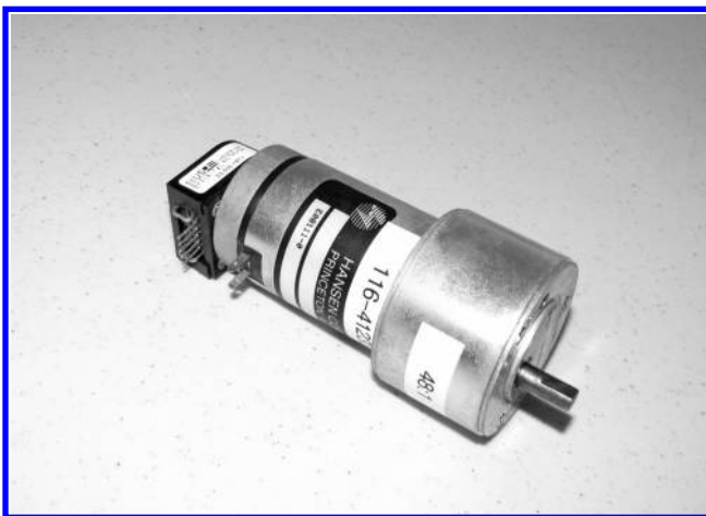
FIGURE 7.16 500-line kit encoder attached to a DC gear motor.
