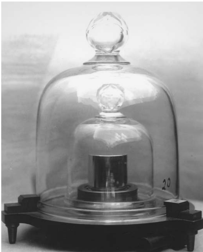
FIGURE 1.2 U.S. kilogram No. 20.
