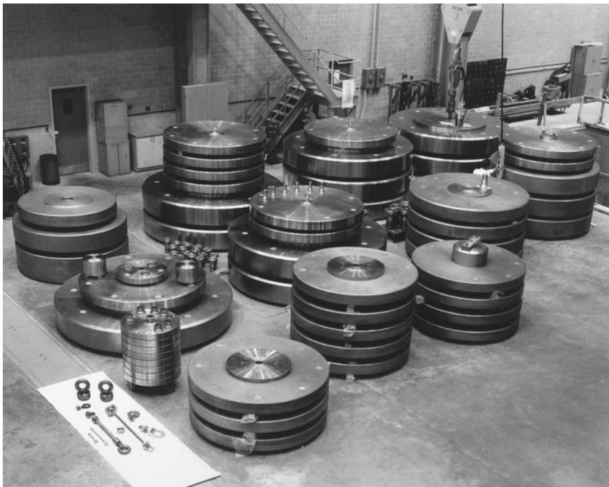
FIGURE 1.5 Large stainless steel weights that when assembled become a deadweight force machine.
