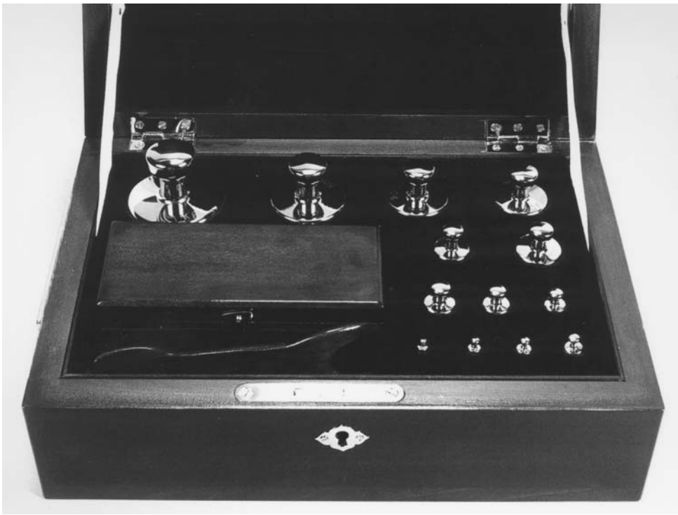
FIGURE 1.4 Stainless steel weight set.
