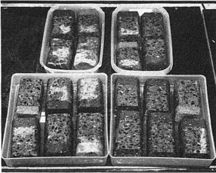
Figure 8. Prepared direct shear specimens.
