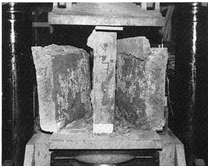
Figure 10. A tested double shear specimen.
