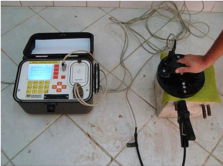
Figure 3. Measurement system used to determine the corrosion current intensity in the reinforced concrete probes.
