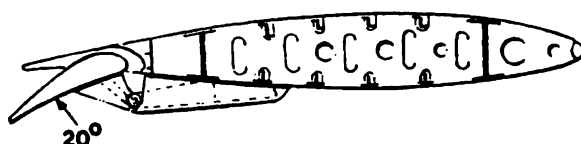
Figure 4.77 Single Slotted Flap Installation FR T-46
