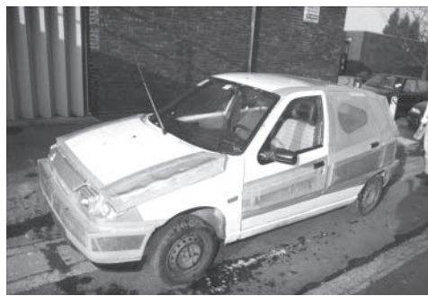
Figure 9.8 One of the camouflaged Fiat Punto prototypes used in the road trials
