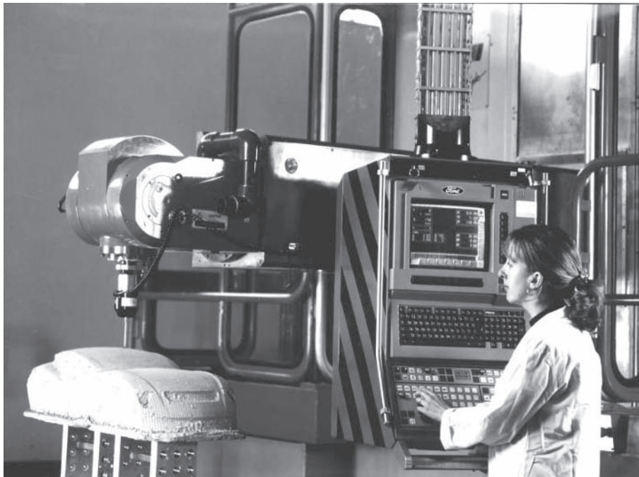
Figure 4.2 Single post system
