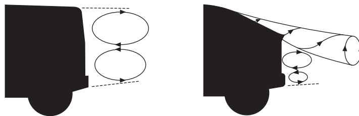
Figure 5.4(a) 'Squareback' large scale flow separation. (b) 'Hatchback/Fastback' vortex generation
