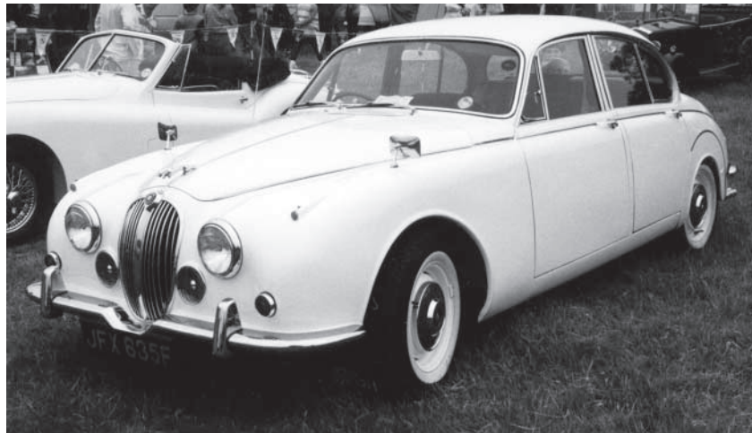
Figure 1.14 The Jaguar 3.4 of the late 'fifties featured all round independent suspension, an unusual feature on a production saloon car at that time
