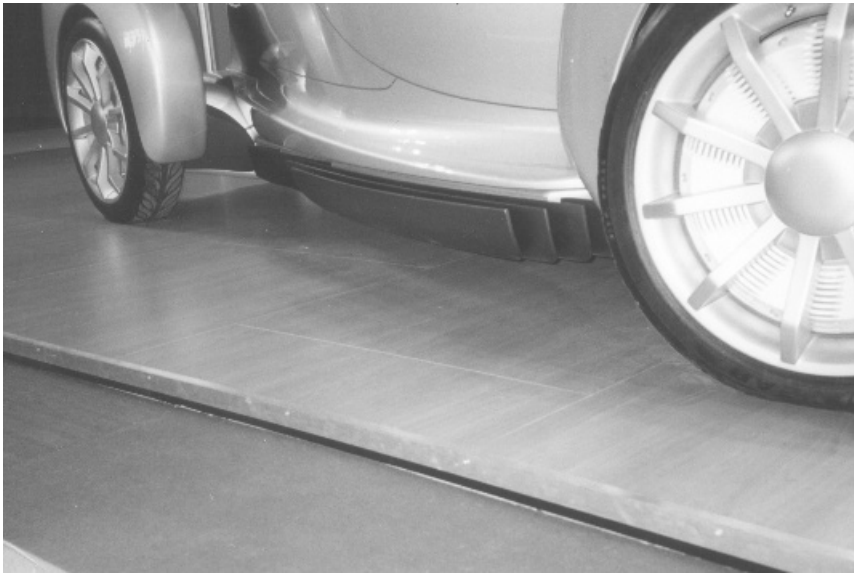
Figure 4.22 Solid metal cooling fins on the side of a GM Hy-wire demonstration fuel cell vehicle
