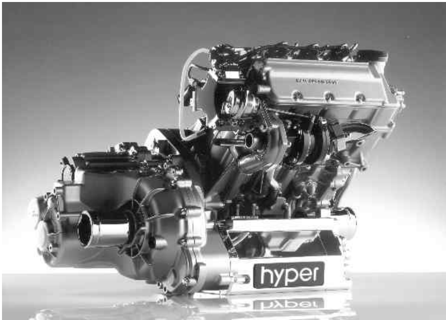
Figure 6.36 Demonstration hybrid diesel/electric power unit installed in a Smart. The motor/generator is the unit marked ‘hyper’ at the base. (Photograph reproduced by kind permission of Micro Compact Car smart GmbH.)
