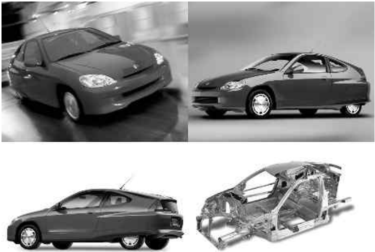
Figure 8.15 Aluminium body from the Honda Insight (Reproduced by kind permission of the Honda Motor Co. Ltd.)
