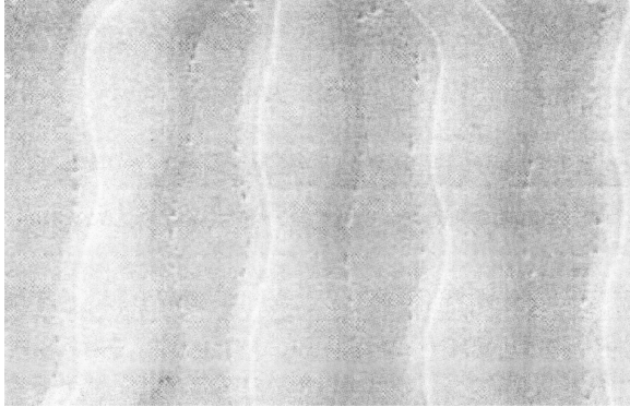
Fig. 3.19. The defects (damages) observed on silicon surface due to excessive stress.
