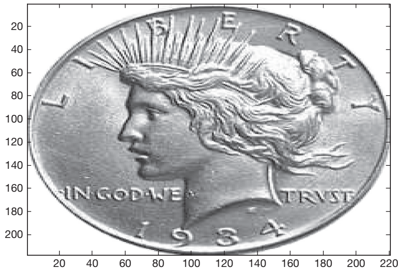
FIGURE 13.9 A JPEG image displayed with image command. Notice that the vertical coordinate increases in the downward axis direction.
