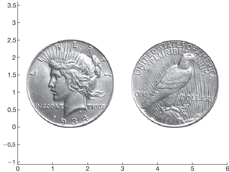
FIGURE 13.11 The front and back coin image objects are positioned on a Cartesian axis by setting their XData and YData properties.
