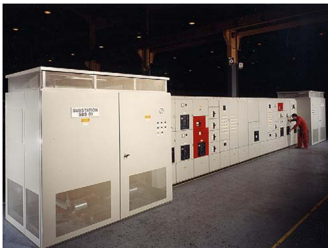
FIGURE 5.4 A sub-station comprising two 1600kVA, 11kV to 415V transformers, incoming and outgoing circuit breakers, fuseswitches controlling outgoing circuits and integral power factor correction (Durham Switchgear Ltd).
