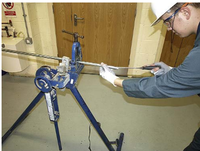
FIGURE 9.8 Conduit should be cut using a hacksaw and after cutting and threading any burrs should be removed using a file.
