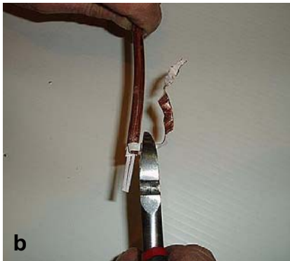
(a) Preparing cable end. Strip cable end by gripping the edge of the sheath between the jaws of side-cutting nippers and twist the cable off in stages, keeping the nippers at about the angle shown. (b) Then proceed in a series of short rips, pulling off the sheath in a spiral.
