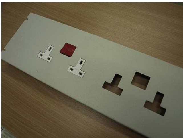
FIGURE 10.2 Shallow sockets can be obtained for fitting to the lid of skirting trunking and trunking manufacturers will punch suitable apertures for the reception of sockets.
