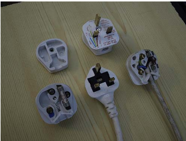
FIGURE 15.6 The 13A plug, for attachment permanently to the appliance for which it will be used, can carry a fuse of suitable rating up to 13A to provide individual protection for that appliance. The plugs shown are of two types. That showing the interior with fuse and cable grip arrangement is available to be fitted to the appliance. The other type (centre) is moulded to the flexible cable in the factory and cannot be subsequently removed. Both types have sleeved pins as required by BS 1363.
