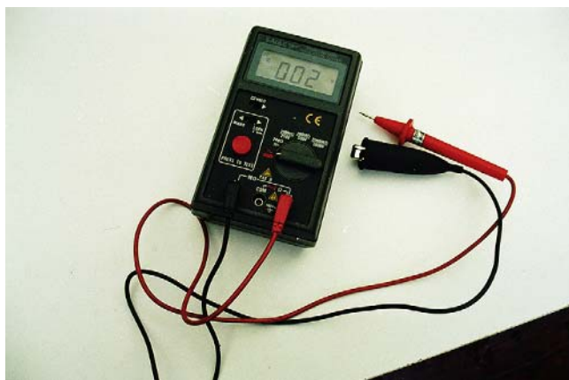
FIGURE 16.4 A 250/500/1000V insulation and continuity tester, with digital display.
