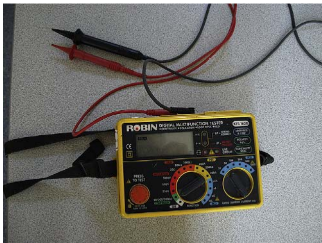
FIGURE 16.5 A battery-operated insulation resistance test instrument operates at 250, 500 or 1000V.
