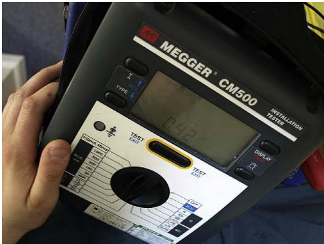
FIGURE 16.9 This digital instrument is capable of testing RCDs. Devices with ratings from 30mA to 1000mA may be tested.
