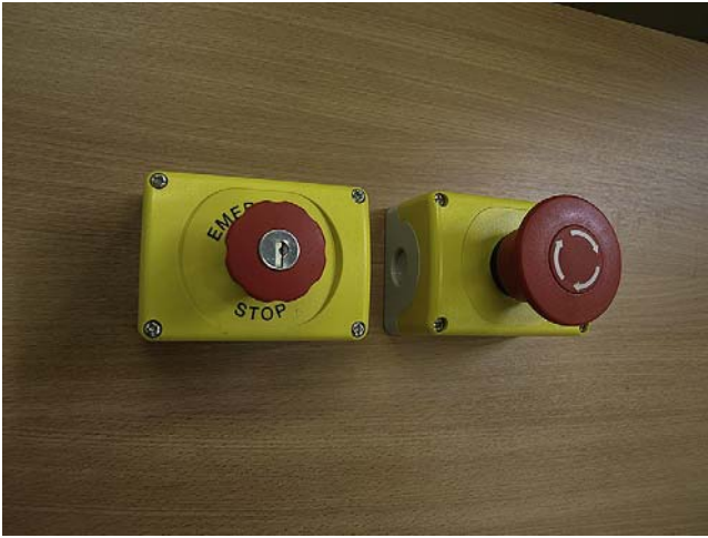
FIGURE 5.25 Emergency stop buttons, here shown with and without a key operated reset facility. The former (shown left) can be used where restoring the power must be carried out by authorised persons.
