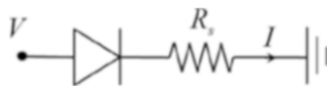
Fig. 11.6 The effect of a finite resistance of the QNRs modeled as a resistance R_s connected in series to the diode
