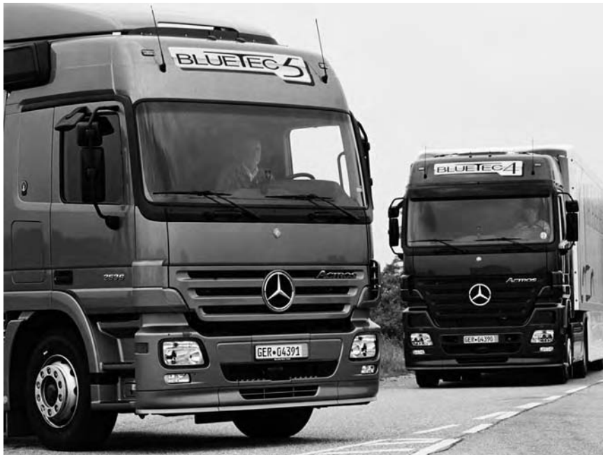
Figure 13.14 BlueTec®-equipped Actros with Euro-4 or Euro-5 emission level and AdBlue® tank
