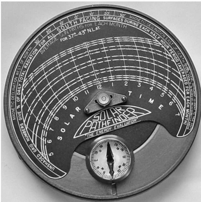
Figure 3.63 Solar Pathfinder platform showing the removable shading graph, the leveling bubble at the center, the triangular holder, and the compass. Photo courtesy of Solar Pathfinder.
