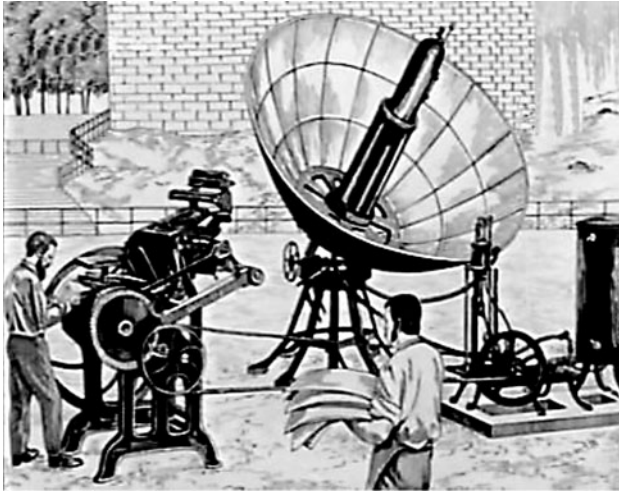
Figure 6.1 Historical use of passive solar energy to power a printing press.
