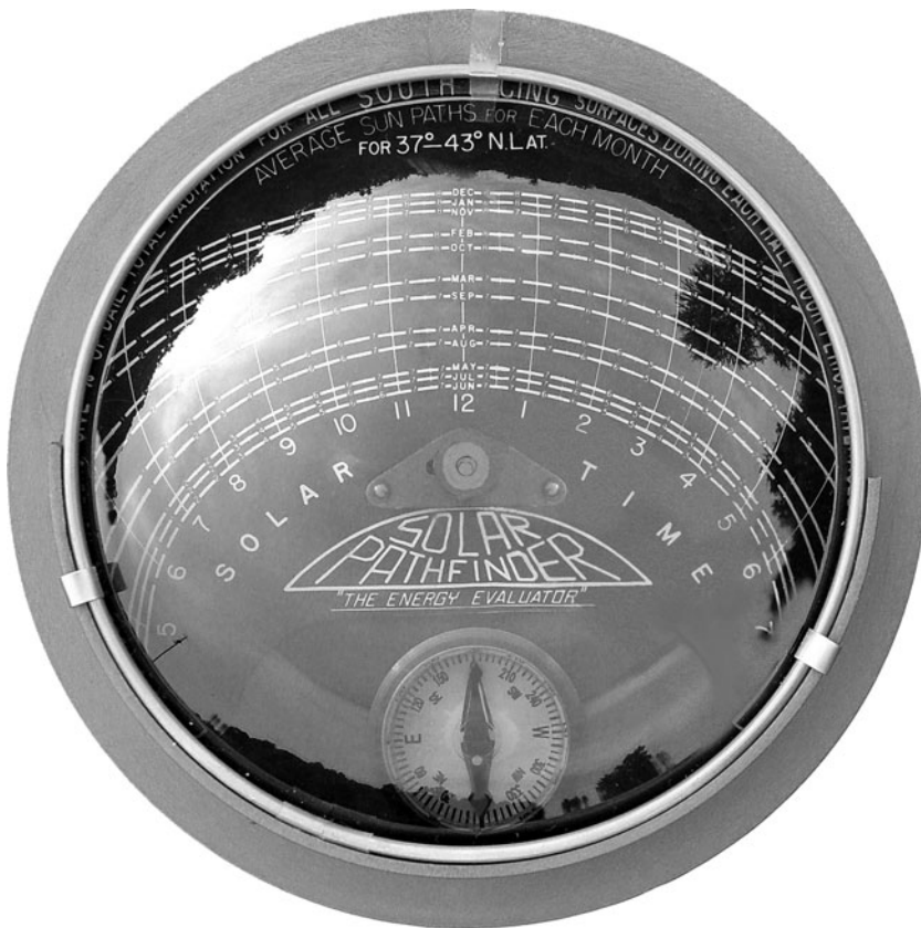
Figure 3.61 Solar Pathfinder semispherical dome showing reflections of surrounding buildings. Photo courtesy of Solar Pathfinder.
