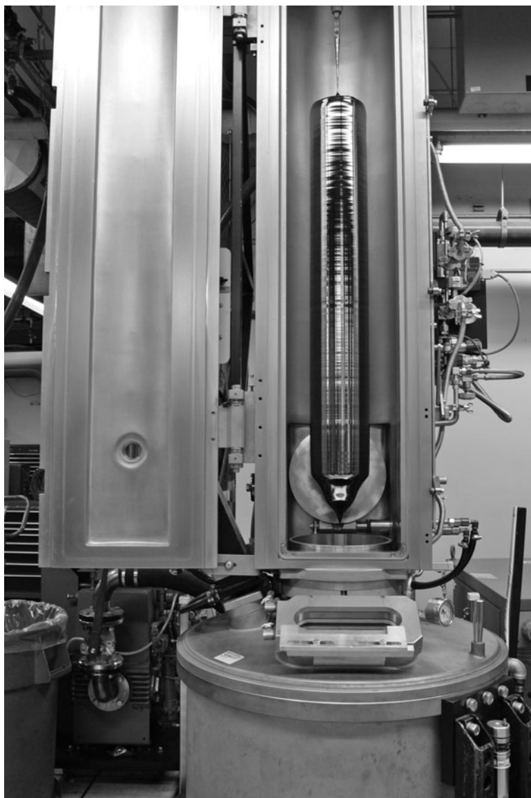
Figure 3.18 Silicon ingot production chamber. Photo courtesy of SolarWorld.
