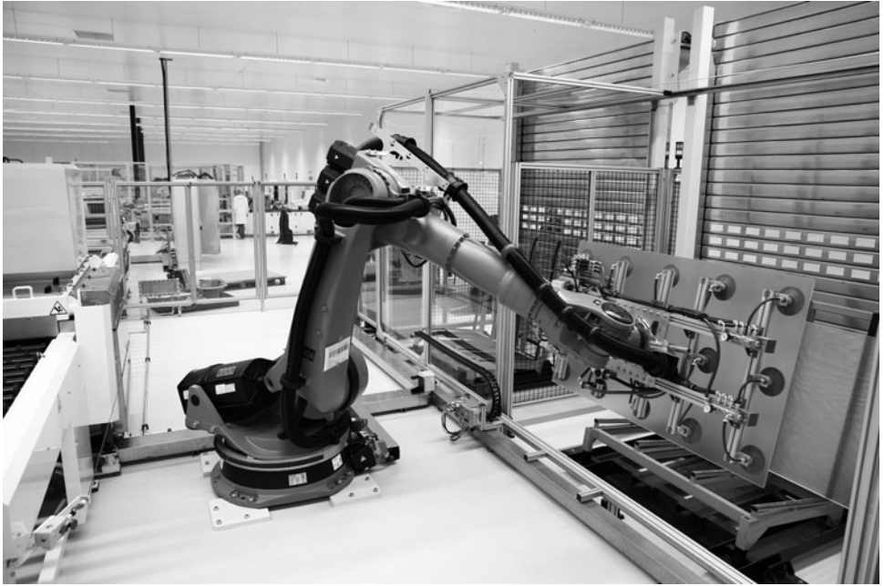
Figure 3.19 A robotic solar power laminator. Photo courtesy of MARTIFER.
