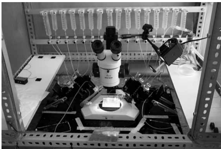
Fig. 2. Inside the cage. Front: the Faraday cage aperture. Middle: the microscope with the recording chamber already positioned and flanked by the two micromanipulators. Rear: 30-mL syringes vertically aligned with the electrovalves of the perfusion system.
