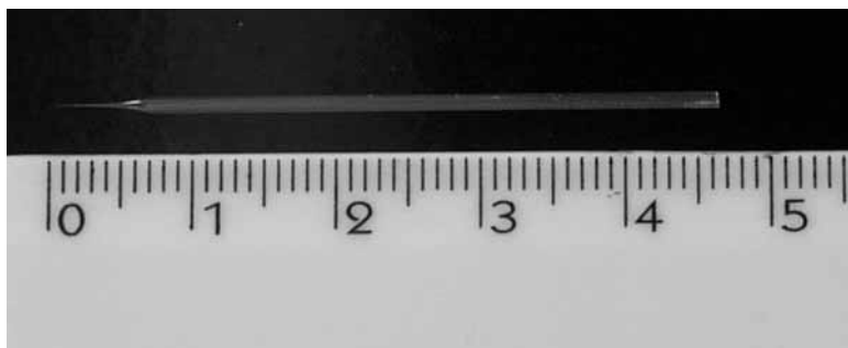
Fig. 5. Pulled glass microelectrode appearance (centimeters).
