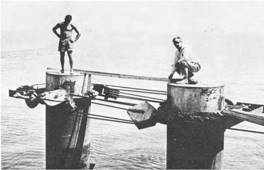
Figure 11.17 Lateral loading test on two steel tubular piles forming part of a breasting dolphin.
