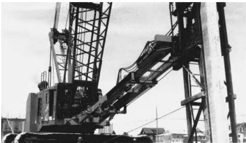
Figure 3.3 ICE 225 spotter with optional front lead rotation (courtesy International Construction Equipment).
