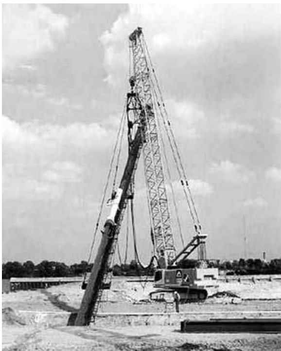
Figure 3.4 Liebherr LRH 400 48 m long swinging leader on HS 885 HD crane (courtesy Liebherr Great Britain Ltd).
