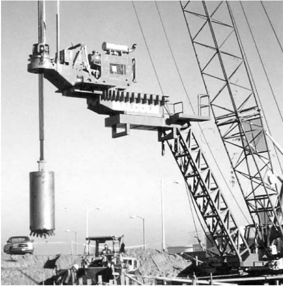
Figure 3.25 Watson 5000 crane attachment power auger on elevated platform on a 40 tonne crane with 200 mm telescopic kelly for installing 2440 mm casings.
