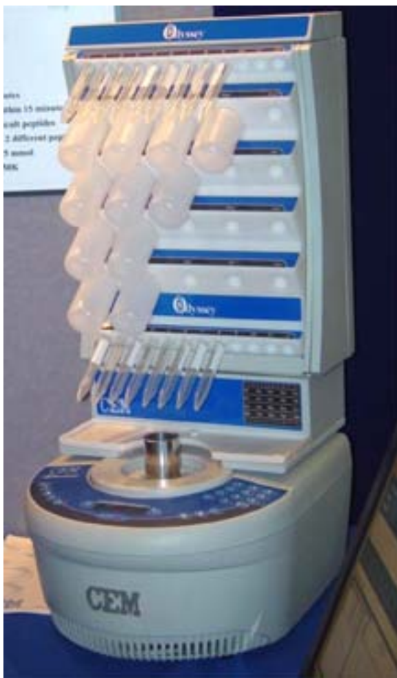
Fig. 7. CEMs Odyssey microwave synthesizer. (Photo by ML.)
