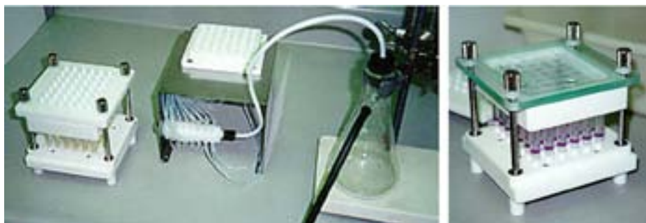
Fig. 2. Multiblock. Arrangement of 42 syringes with multistoppers and washing station. Left—Multiblock with upper and lower multistopper attached to it for coupling reaction next to the washing station. Right—Multiblock with cover used for resin distribution. (Photo by ML.)
