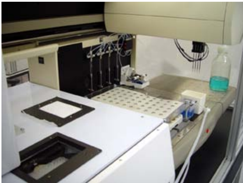
Fig. 9. View of the deck of peptide synthesizer utilizing tilted centrifugation principle. (Photo by ML.)
