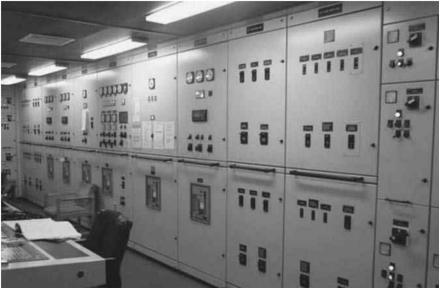
FIGURE 8.13 Typical main switchboard on large cargo ship. (From Raul Osgian, U.S. Merchant Marine Academy.)
