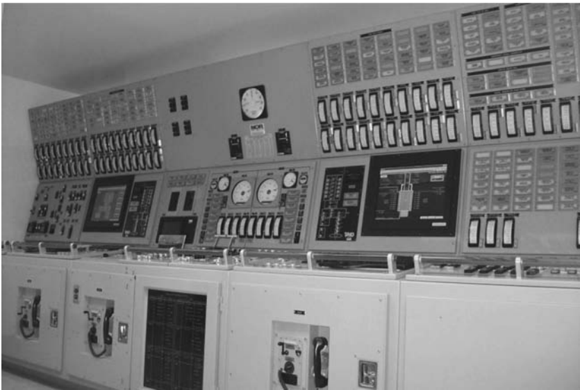
FIGURE 2.10 Ship simulator for a U.S. Navy oil tanker (from Captain Elwood Baumgart, U.S. Merchant Marine Academy).
