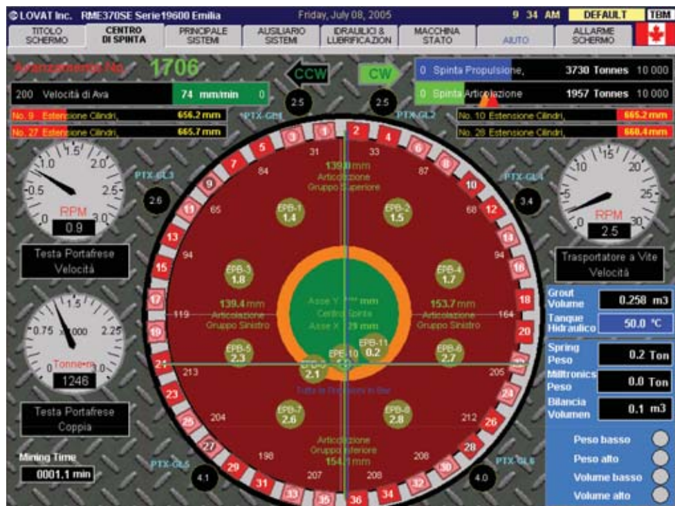
Figure 6.17 Screen display of the control parameters during excavation by EPBS.
