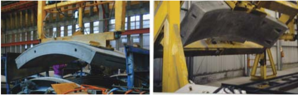
Figure 5.79 Segment extraction from mould and rotation.
