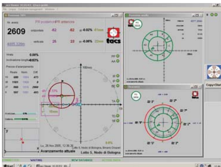
Figure 8.60 The TACS guidance system screen.
