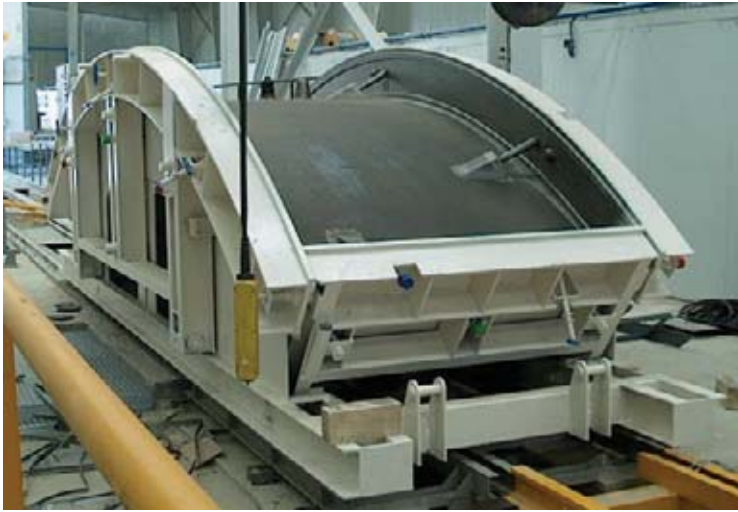
Figure 5.76 Example of a typical mould.
