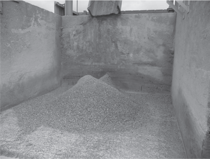
Figure 17.5 Recovered aggregates; Cemex plant at Ivry.
