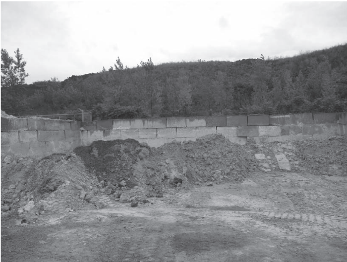
Figure 17.21 Hardened sludge before its elimination; Demix Béton plant.
