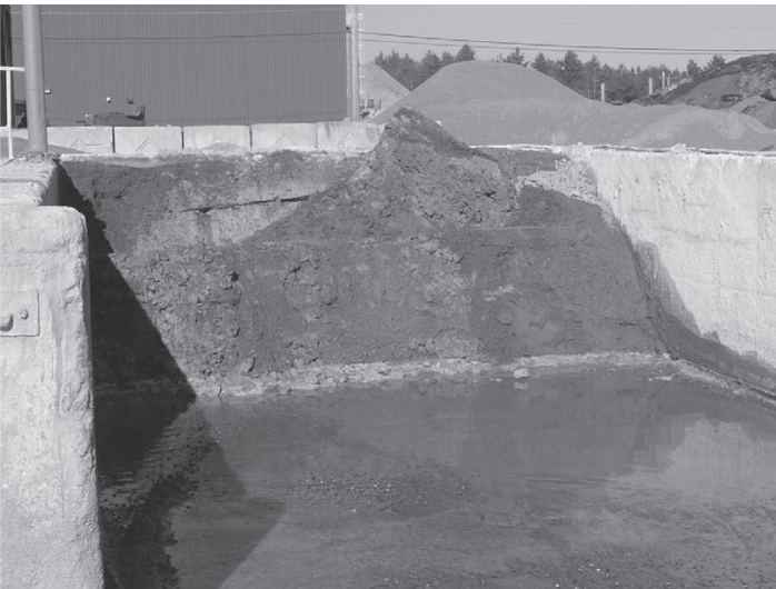
Figure 17.23 Hardened sludge before its elimination; Béton Memphré plant.
