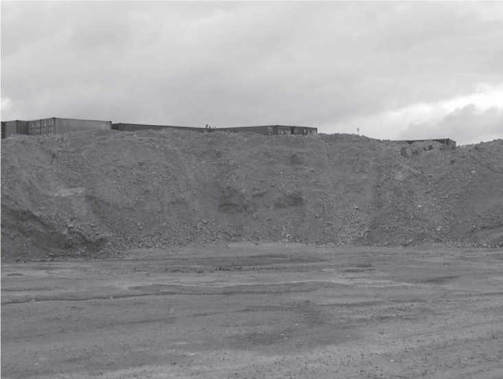
Figure 17.17 Crushed demolition concrete; Demix Béton plant.
