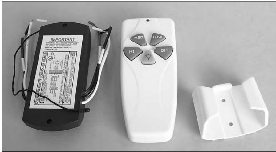
Figure 5-1: This manufacturer-supplied remote controls a ceiling fan.
