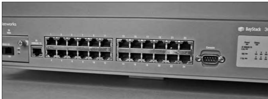
Figure 12-3: Switches make more efficient use of network bandwidth than hubs.
