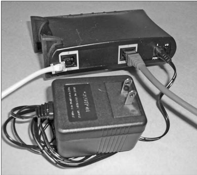
Figure 12-1: View of typical DSL modem connection ports.
