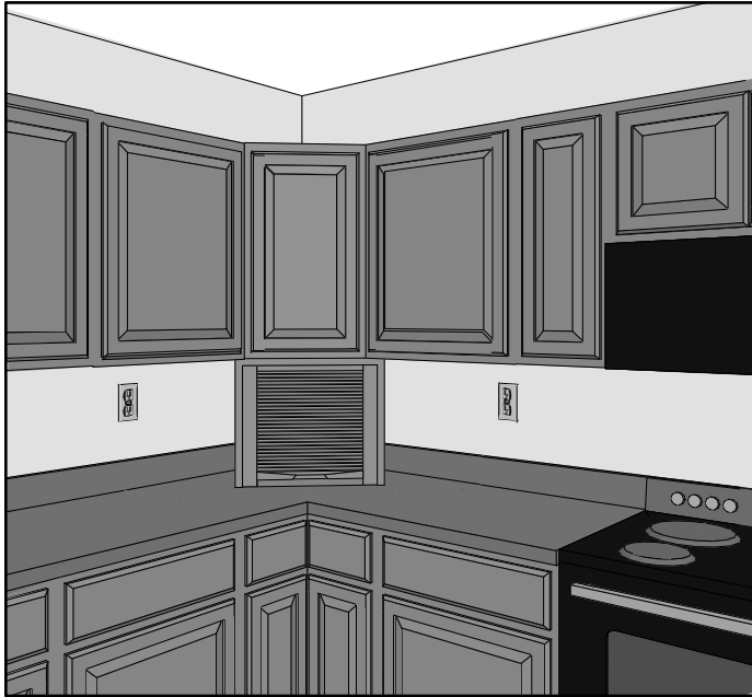
Figure 3-3: An appliance garage.
