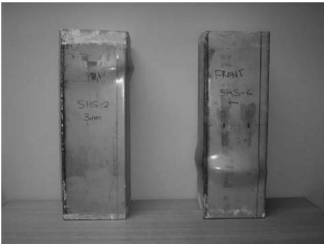
Figure 3.22 Local buckling of rectangular CFST short columns.
