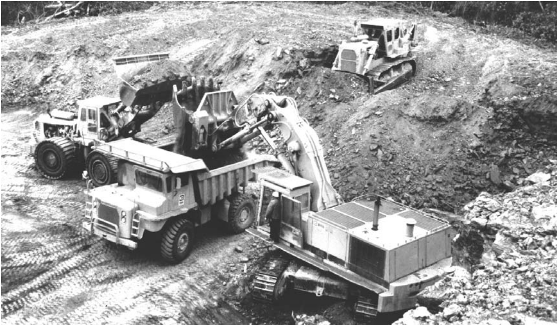
Fig. 13.6 Hydraulic shovel loads off-highway dump truck. (Caterpillar Tractor Co.)
