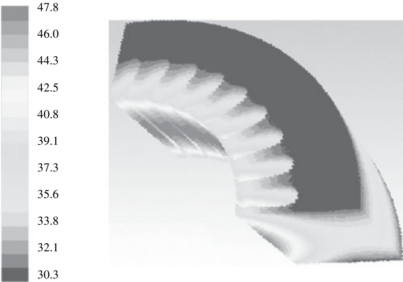
Figure 10.18 Temperature distribution in stator.
