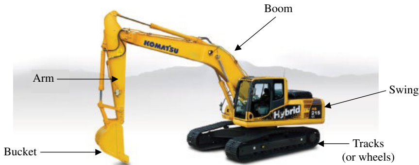
Figure 6.10 A typical excavator with parts labeled. Source: Reproduced with Courtesy of Komatsu.
