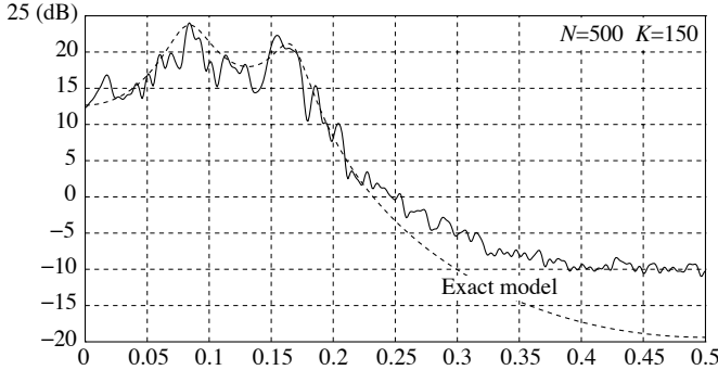
Figure 9.2 – Non-parametric estimation of an AR-4 spectrum based on K = 150 estimates of the covariance coefficients. The length of the sample is N = 500 . The window used is the Bartlett window
