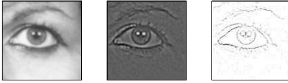
Figure 6.22 – Results of thresholding and of the search for local maxima
