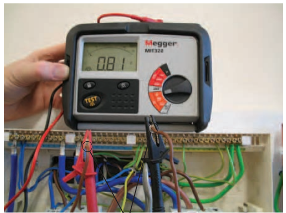
Ends of phase conductor
