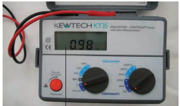
Low resistance reading
