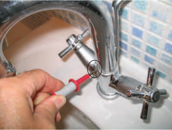
Probe on solid metal part of tap
