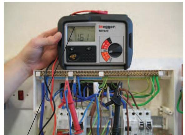
Resistance double that of phase conductor P2 P1 joined to N2 N1
