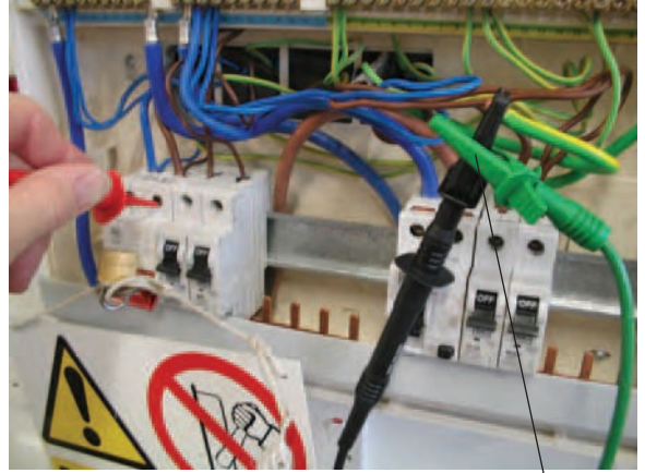
Connections for 3-lead instrument Leads joined
