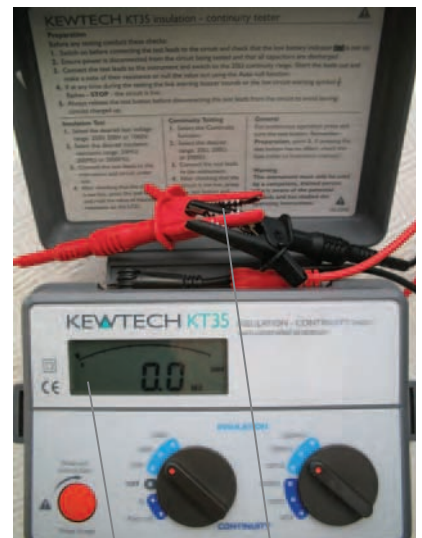
Closed circuit Leads connected
