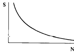
Fig. 2b. S-N no endurance limit
