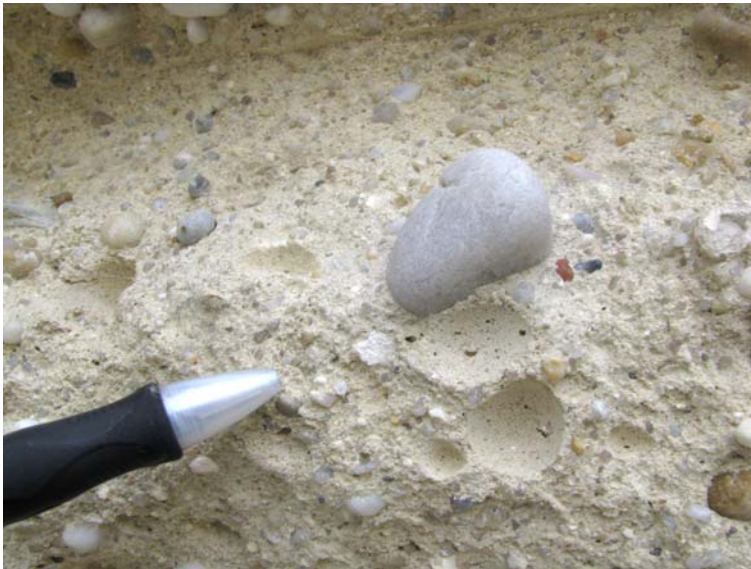
Figure 6. Heterogeneous erosive behaviour of artificial material due to heterogeneous constituents.
