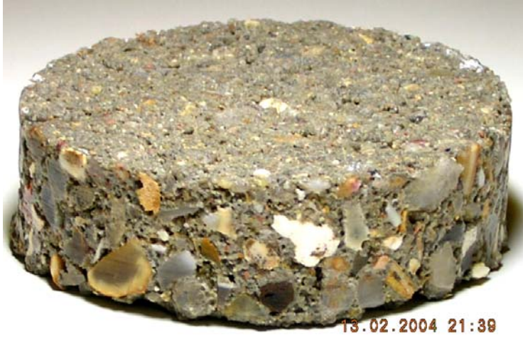
Figure 1. Photo of the sample cut off from the hollow block.
