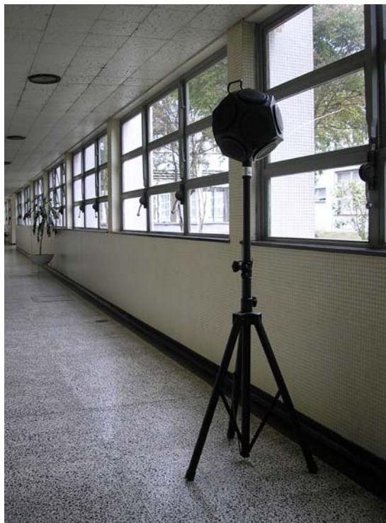
Figure 5. Omnidirectional Sound Source.
