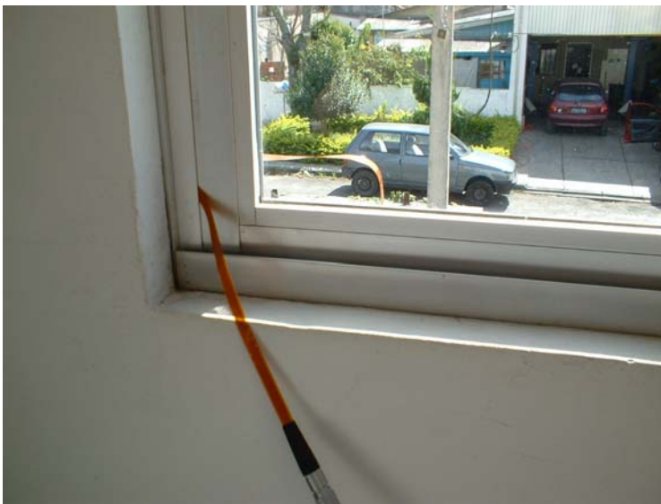
Figure 2. Use of a flat cable in measurements of the sound insulation of façades.
