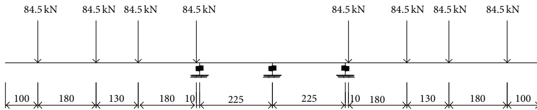
FIGURE 21: Load spread schematic diagram of model two.
