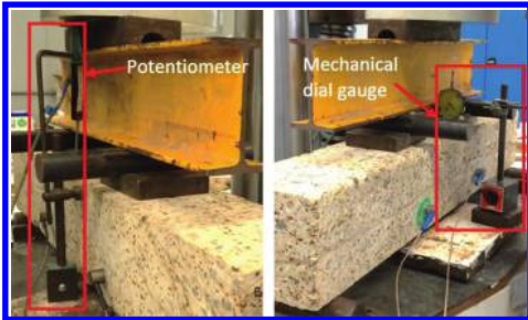
Figure 7. Testing equipment of beam 1 and 2.
