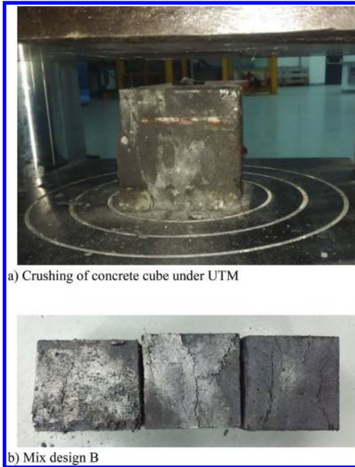
Figure 5. Failure mode of cube specimens.
