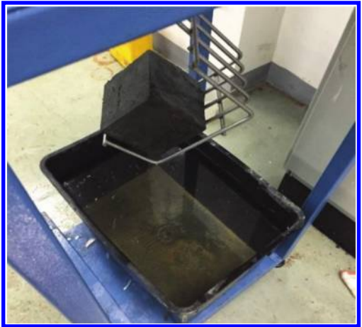
Figure 3. Buoyance balance for density measurement.
