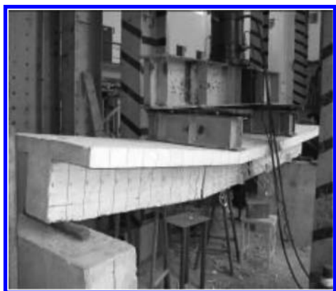
Figure 7. Overall deformation of SCB-2.
