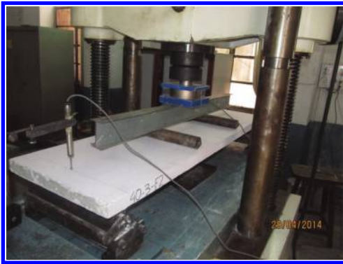
Figure 1. Setup for flexural test.
