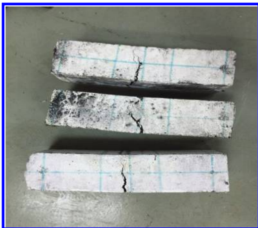
Figure 8. Failure mode of specimens (side view).
