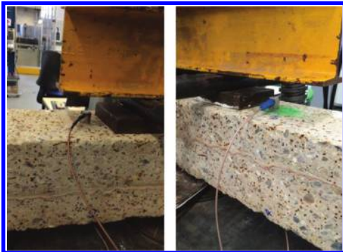
Figure 8. Testing equipment of beam 3.
