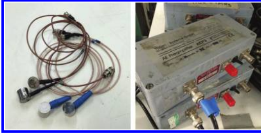
Figure 3. Four AE sensors and preamplifiers used in the experiment.
