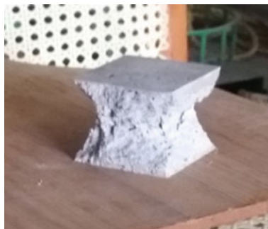
Fig. 3 Typical failure pattern in mortar cube specimen
