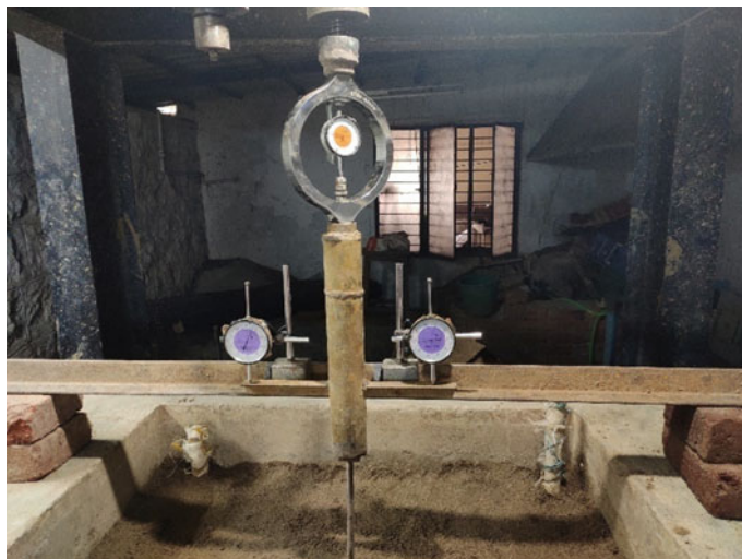
Fig. 3 Test setup for laboratory-scale load test
