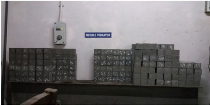
Fig. 2 Ambient air curing of the specimens
