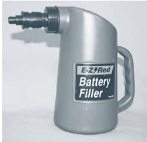
Figure 7.14. Battery Filler Bottle. Battery filler bottles work well for systems in which batteries are accessible. Credit: Dan Chiras.
