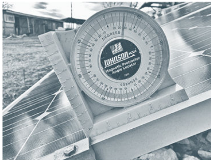
Figure 8.11. Magnetic Angle Finder. This inexpensive device is used to check the angle of roofs and arrays. Credit: Dan Chiras.
