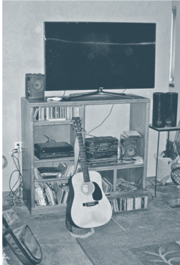
Figure 4.2. Phantom Load. This superefficient, 50-inch Samsung flat-screen television uses only 60 to 130 watts when operating. Because of the instant-on feature, however, it continues to draw 8 watts when turned off. The satellite receiver attached to the TV uses 26 watts when operating and 24 watts when turned off. To save energy, homeowners can plug electronics like this into power strips that are shut off when the unit is not on. Or, a homeowner can install an outlet controlled by a switch; however, these must be installed during construction. Credit: Dan Chiras.
