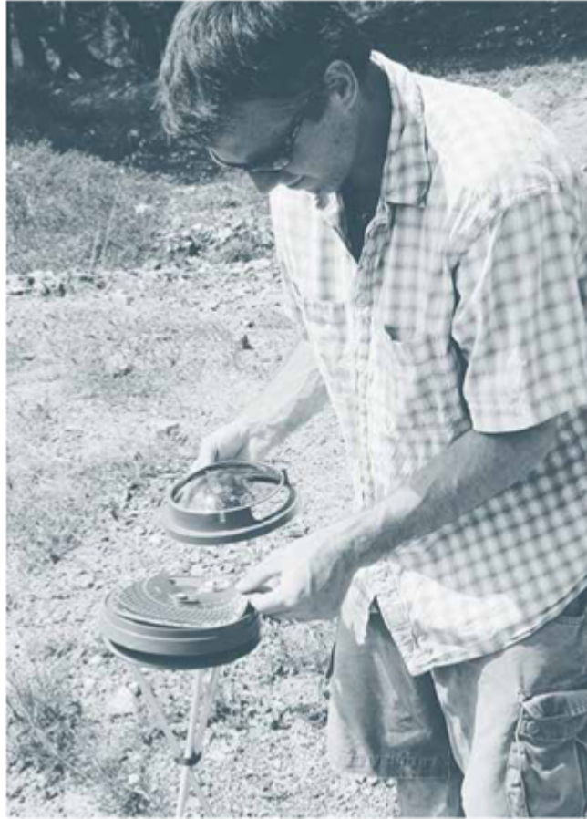
Figure 4.6. Solar Pathfinder. This device allows solar site assessors and installers to assess shading at potential sites for PV systems, helping them select the best possible site to install an array. Credit: Shawn Schreiner.
