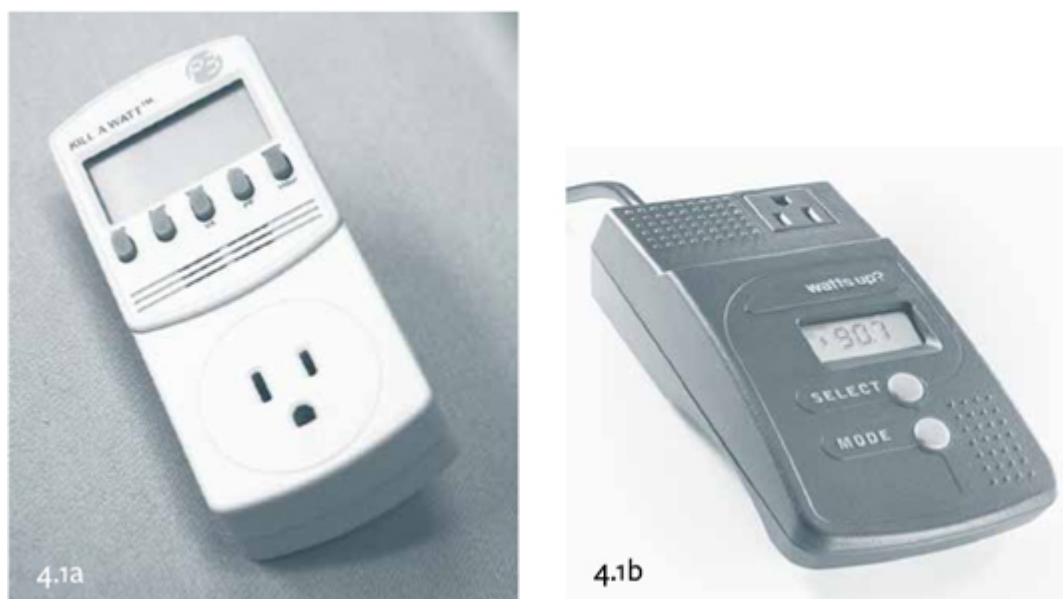
Figure 4.1. (a) The Kill A Watt and (b) Watts Up? meters can be used to measure wattage of household appliances and electronic devices. Of the two, the Watts Up? is the more sensitive and allows for measurement of tiny phantom loads as well. Credit: (a) Dan Chiras, (b) Electronic Educational Devices.
