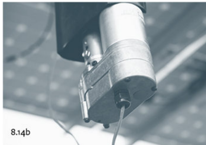
Figure 8.14. (a) Motor That Adjusts Azimuth Angle. This motor sits atop the pole and adjusts the azimuth angle of the array to track the Sun on its east-to-west path across the sky. (b) Motor That Adjusts Tilt Angle. A smaller electric motor adjusts the tilt angle of the array to accommodate the ever-changing altitude angle of the Sun. Credit: Dan Chiras.
