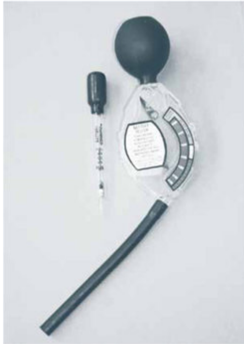
Figure 7.11. Hydrometer. Hydrometers like these can be used to test the condition of battery acid, one cell at a time, a process that is time consuming and boring. They measure the specific gravity, which is determined by the concentration of sulfuric acid, as explained in the text. Be careful when you do this so you don't splash sulfuric acid on yourself. Credit: Dan Chiras.
