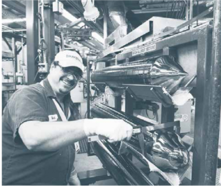
Figure 3.2. Silicon Ingot. This ingot is a huge crystal of silicon that is sliced to make monocrystalline PV cells. Credit: SolarWorld.
