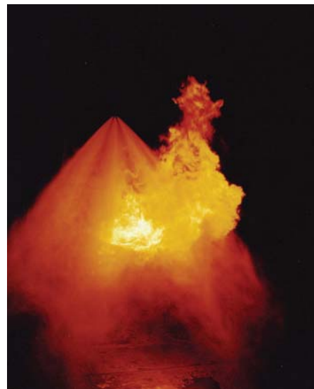
Figure 9.67 High pressure water mist system in operation
