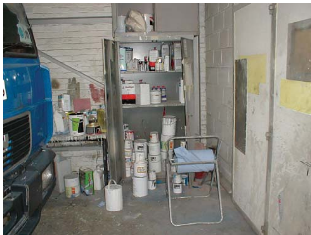
Figure 8.5 Poor storage arrangements for flammable materials
