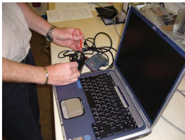
Figure 8.13 Portable appliance testing
