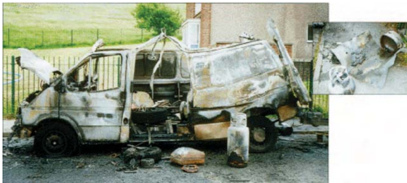
Figure 8.4 Van fire involving cylinders
