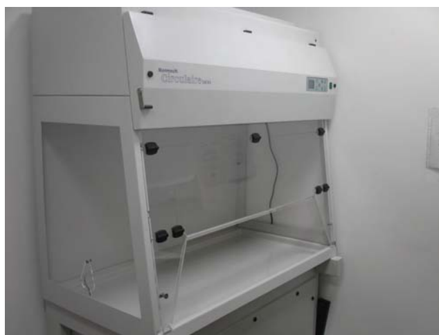
Figure 8.23 Example of a fume cupboard
