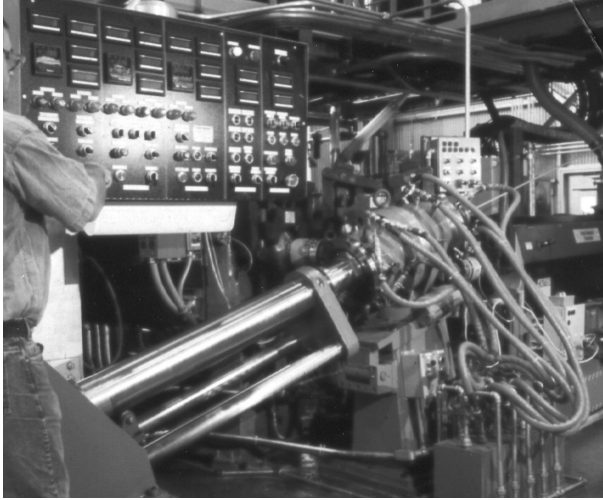
FIGURE 11.3 Crosshead and extruders.
