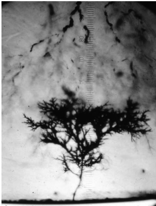
FIGURE 19.12 Electrical tree in a water tree. Photo by W. A. Thue.
