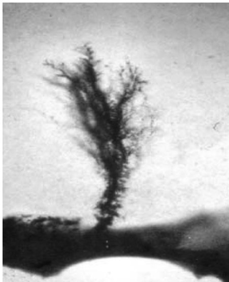
FIGURE 19.8 Bush tree growing from a shield (hence vented). Photo by W. A. Thue.
