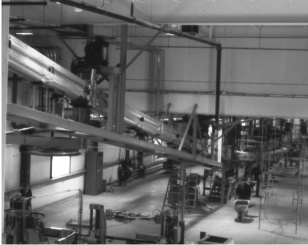
FIGURE 11.4 Curing section of dry cure CV line.
