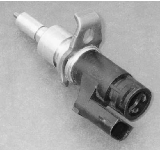
Figure 12-37 VSS used on applications that retain a speedometer cable to operate a mechanical speedometer. © Cengage Learning 2012
