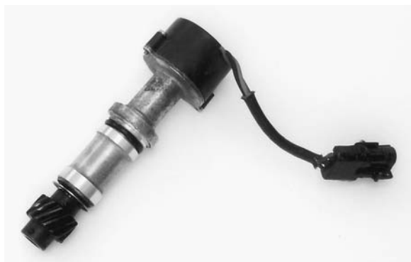
Figure 10–49 Hall effect camshaft position sensor that mounts in the distributor hole. © Cengage Learning 2012
