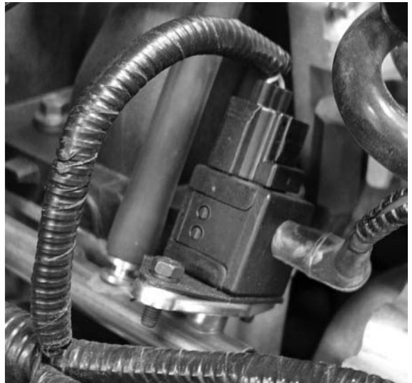
Figure 13-11 This fuel rail pressure sensor monitors the difference between fuel rail pressure and manifold absolute pressure. © Cengage Learning 2012
