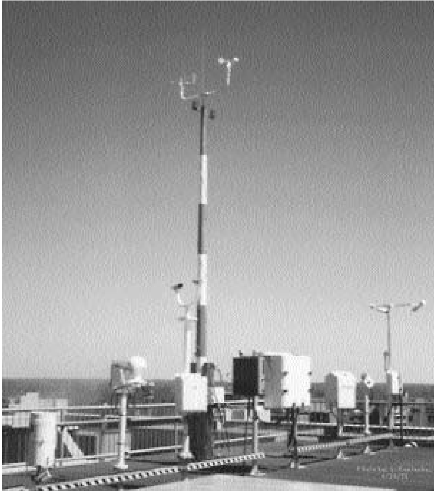
Figure 4-40. ASOS-3 system. (Source: FAA)
