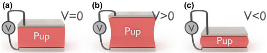
Fig. 6.1 The CPE explained: without bias applied the material rests in its initial position, a For a given positive bias applied, the material expands, b while for a negative bias, c MUT contracts
