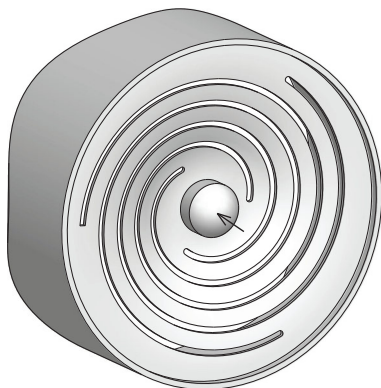
Figure 8-6 Triple spiral frictionless flexure for guiding axial displacement.
