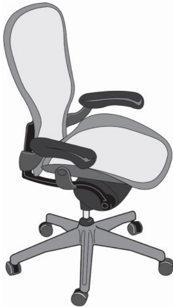
Figure 3-17 Office chair with five legs shows elastic constraint design.
