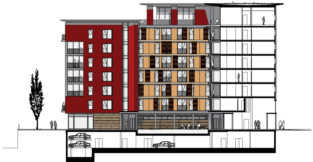
Sectional elevation through section A of the building looking eastwards from the courtyard
