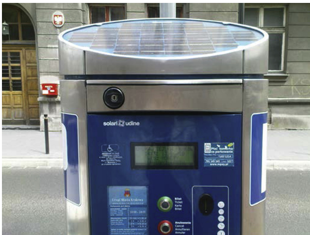
FIGURE 7.23 A standalone PV system.
