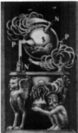
Figure 5-8a. Hero's reaction turbine.
