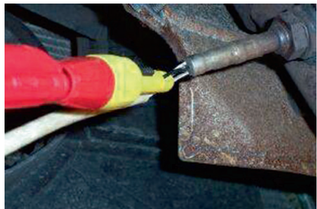
Figure 4.23 Titania knock sensor in position
