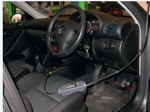
Figure 3.30 Connect the serial lead to the diagnostic socket
