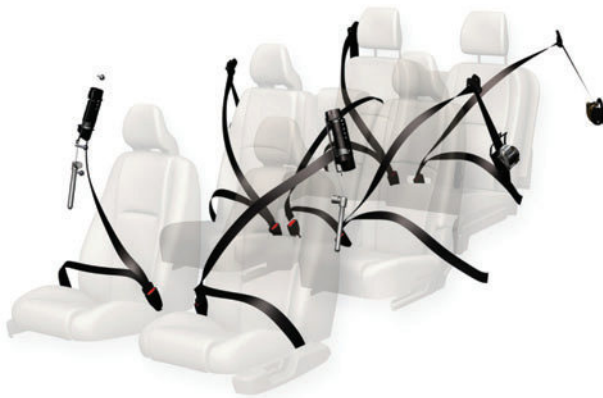
Figure 8.88 Seat belts and tensioner (Source: Volvo Media)
