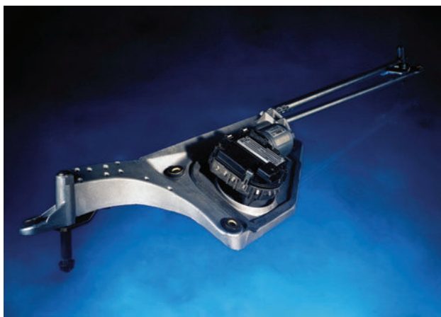
Figure 8.46 Reversible wiper motor and drive linkage (Source: Bosch Media)
