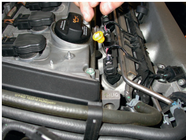
Figure 2.12 Test the voltage by back probing a connector with care
