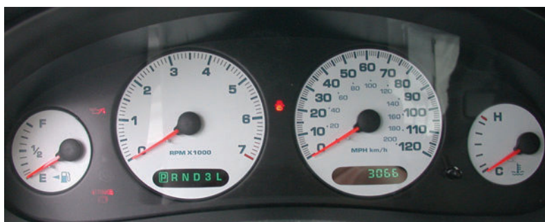
Figure 8.68 Instrument display combining analogue and digital displays
