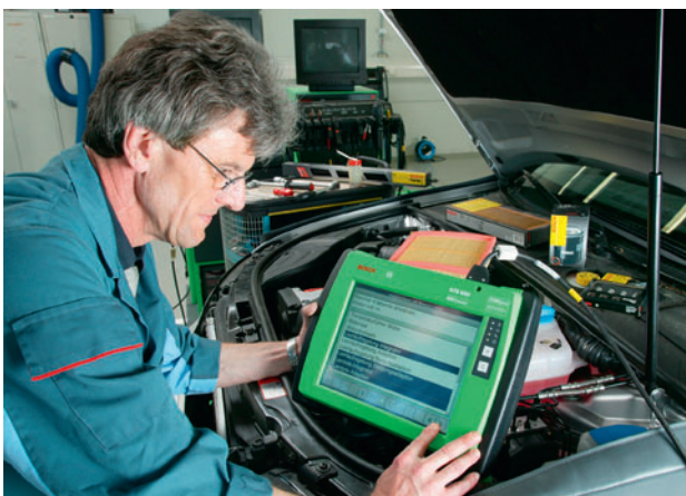
Figure 3.28 Diagnostic system in use (Source: Bosch Media)
