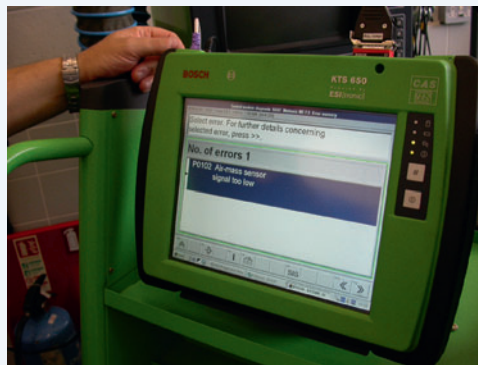
Figure 3.32 Take a readout from the control unit memory (DTC display)
