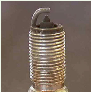
Figure 6.35 Carbon fouled (platinum plug)
