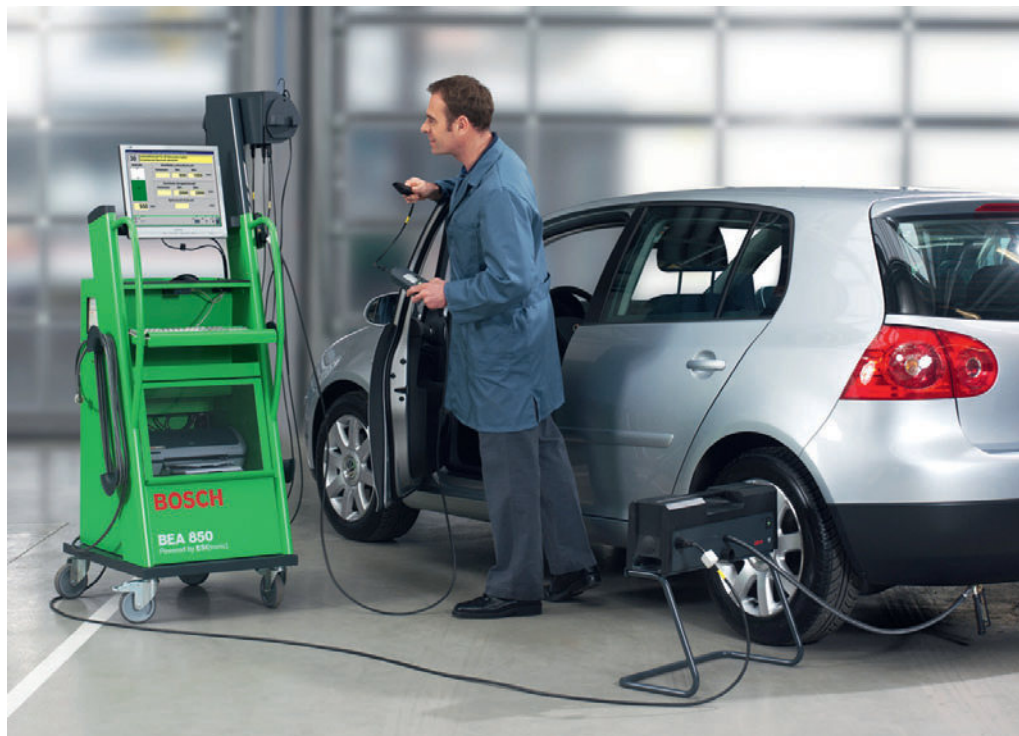
Figure 6.18 Exhaust gas analyser
