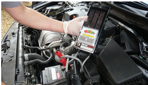
Figure 6.90 A high-rate discharge tester can indicate battery state-of-health, but still relies on the skill and judgement of the technician. In addition, there are several health and safety-related issues to this approach! Note the tester in the picture is a fixed load, and not really suitable for the battery shown (Source: www.autoelex.co.uk )
