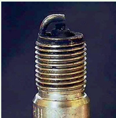
Figure 6.32 Carbon fouled (standard plug)
