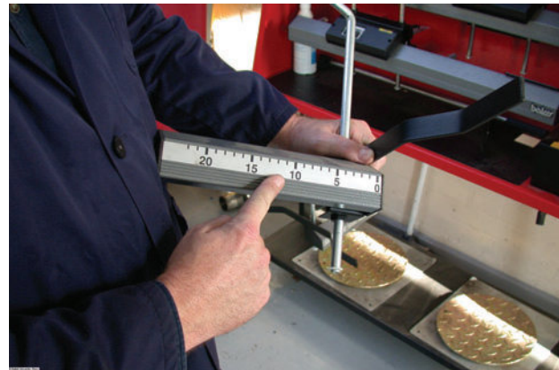
Figure 7.27 Scale to show angle of wheels
