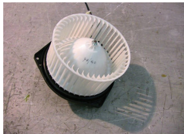
Figure 8.73 Blower motor and fan
