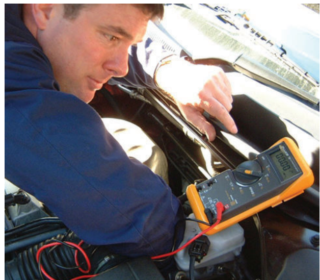
Figure 8.78 Circuit voltage testing
