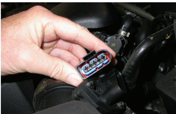
Figure 6.68 Airflow meter under test
