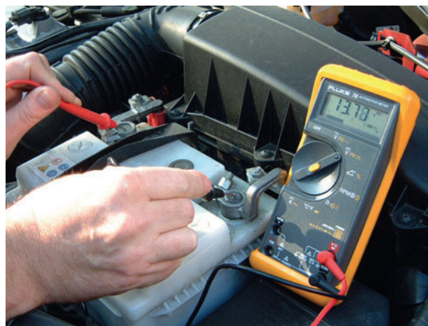
Figure 6.88 Checking battery voltage. In this case, the engine had just been switched off so the reading shows a 'surface charge'
