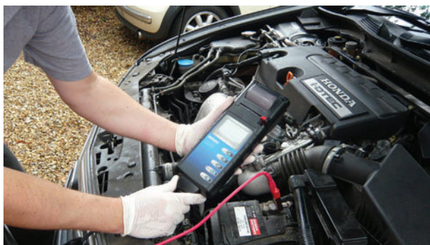
Figure 6.91 Intelligent, digital battery testers are much safer and more appropriate for testing modern battery technology (Source: www.autoelex.co.uk )
