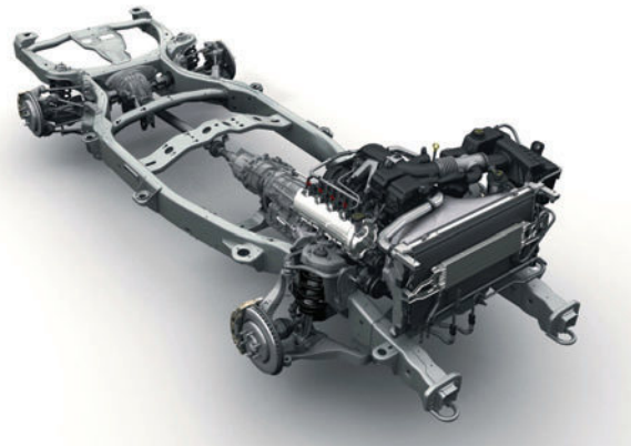
Figure 9.6 4 WD transmission layout (Source: Ford Media)
