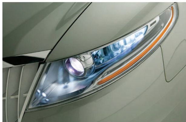
Figure 8.27 Adaptive lighting using LEDs
