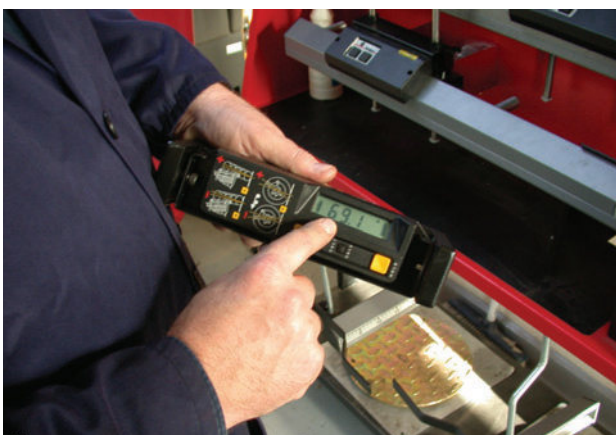
Figure 7.26 Laser alignment systems give digital readouts
