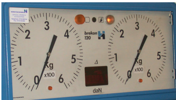
Figure 7.6 Gauges on a rolling road brake tester
