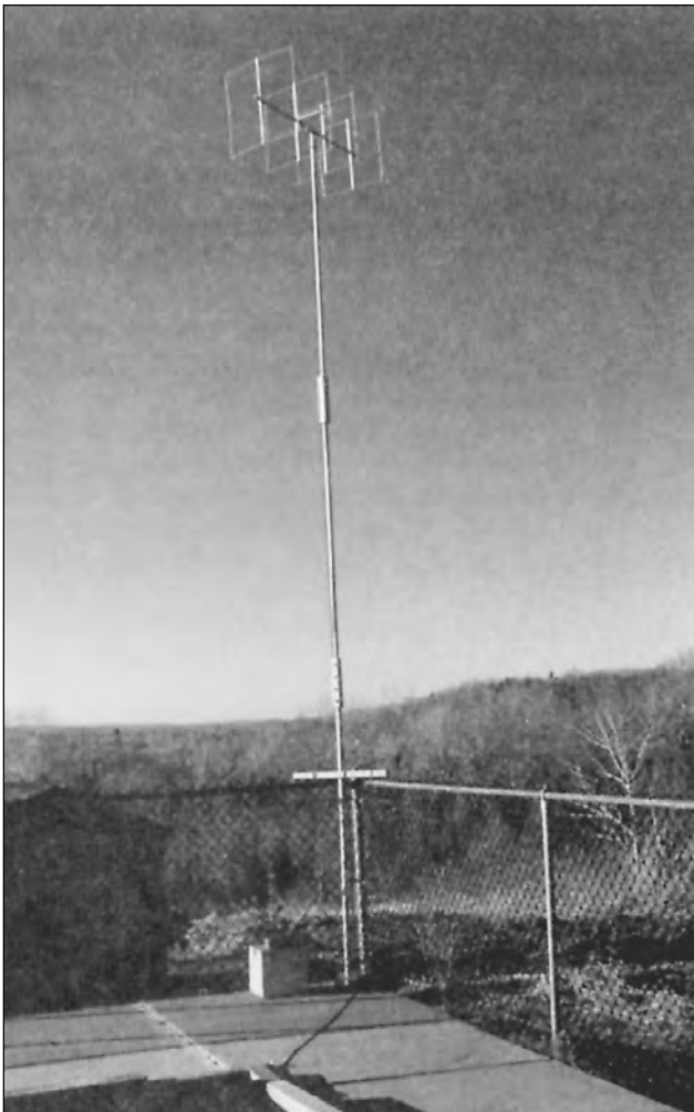
Fig 48—The 4-element 144-MHz portable quad, assembled and ready for operation. Sections of clothes-closet poles joined with pine strips make up the mast. (Photo by Adwin Rusczek, W1MPO)
