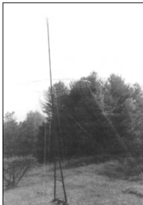
Fig 42—Photo of W8NWF’s original A-frame mounted HF discone.
