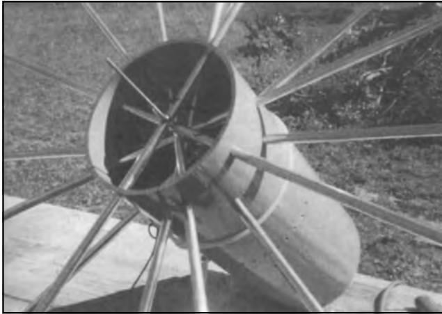
Fig 46 —Photo showing details of the hub assembly for the large dish, including the threaded brass rod that connects the radial spreaders together. The 10-inch PVC pipe is drilled to accommodate the radial spreaders. Each spreader is reinforced with a three-foot long wooden dowel inside for crush resistance. Note the row of holes drilled below the lowest spreader. Each of the 36 cone wire passes through one of these holes.
