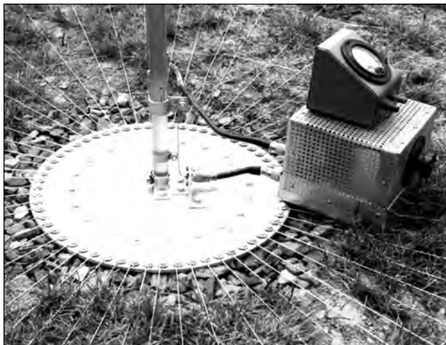
Fig 45—Base of the vertical antenna showing the 60 radial wires. The aluminum disc is 15 inches in diameter and \frac{1}{4} inches thick. Sixty tapped holes for \frac{1}{4} -20 aluminum hex-head bolts form the outer ring and 20 form the inner ring. The inner bolts were used for performance comparisons with more than 60 radials. The insulator is polystyrene material (phenolic or Plexiglas suitable) with a 1-inch diameter. Also shown is the impedance bridge used for measuring input resistance.
