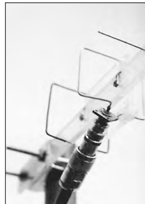
Fig 58 —A view of the 10-element version of the 1296-MHz Quagi. It is mounted on a 30-inch Plexiglas boom with a 3 × 3-inch square of Plexiglas to support the driven element and reflector. Note how the driven element is attached to a standard UG-290 BNC connector. The elements are held in place with silicone sealing compound.
