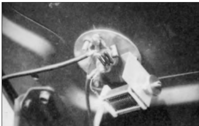
Fig 30 —Details of the matching network located at the base of the antenna inside the vehicle. The mica capacitors are visible at the center. The coaxial stub used to switch them in and out of the circuit comes in from the left, and the feed line exits toward the bottom of the photo.
