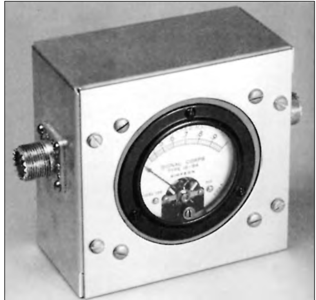
Fig 2—A convenient method of mounting an RF ammeter for use in a coaxial line. This is a metal-case instrument mounted on a thin bakelite panel. The cutout in the metal clears the edge of the meter by about \frac{1}{8} inch.
