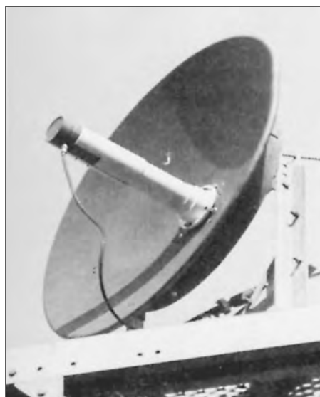
Fig 20—Coffee-can 2304-MHz feed described in text and Fig 19 mounted on a 4-foot dish.
