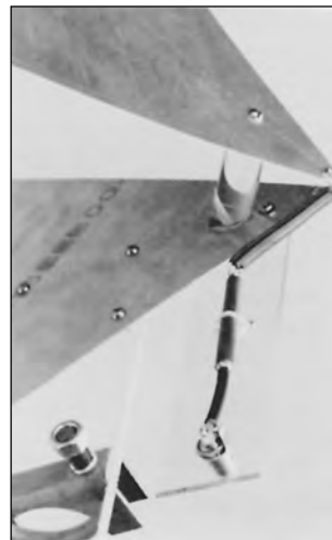
Fig 15—An experimental two-sided pyramidal horn constructed in the ARRL laboratory. A pair of muffer clamps allows mounting the antenna on a mast. This model has sheet-aluminum sides, although window screen would work as well. Temporary elements could be made from cardboard covered with aluminum foil. The horizontal spreaders are Plexiglas rod. Oriented as shown here, the antenna radiates horizontally polarized waves.
