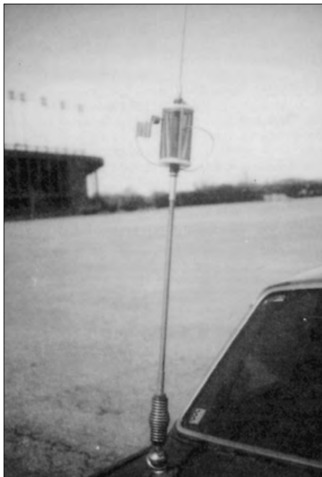
Fig 31 —This photo shows the antenna mounted on the trunk of a car. The structure is somewhat cumbersome, so it is guyed appropriately.
