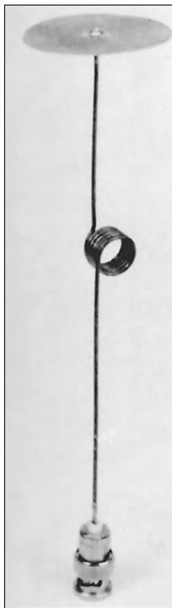
Fig 46—This 144-MHz antenna uses a combination of top and center loading. It offers low construction cost and improved efficiency over continuously loaded rubber-duddy antennas.
