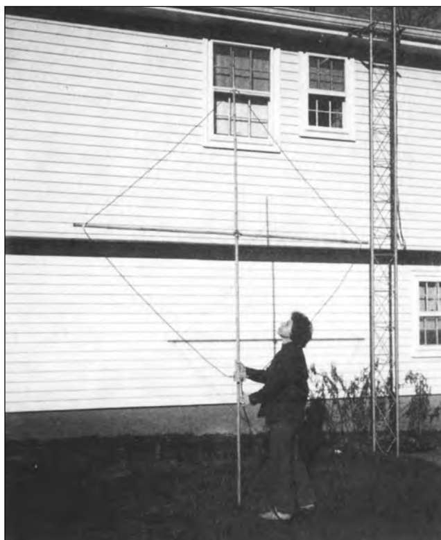
Fig 33—Jean DeMaw, W1CKK, tests the 1.8-MHz shielded loop. Bamboo cross arms are used to support the antenna.
