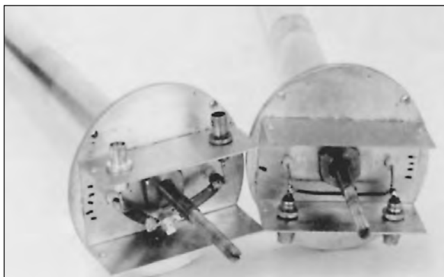
Fig 25 —Two of the center conductor and top plate assemblies. In the assembly at the left, C1 is visible just below the tuning shaft, mounted by short straps made from sheet copper. The assembly on the right has L1 in place between the BNC connectors. The Miniboxes are fastened to the top plate by a single large nut in these units. Using screws through the Minibox into the top plate, as described in the text, is preferred.
