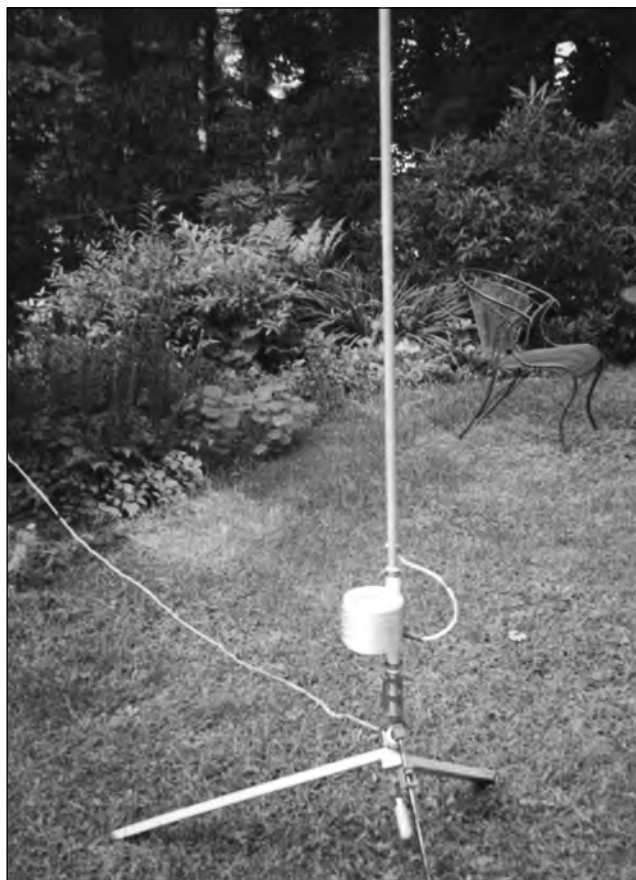
Fig 7— The flagpole bracket that supports the tubing elements is clamped to the long carpenter's clamp, but insulated from it by a small section of 1-inch PVC pipe. A coax connector is mounted to the bracket and the spool of wire is attached to the coax connector.
