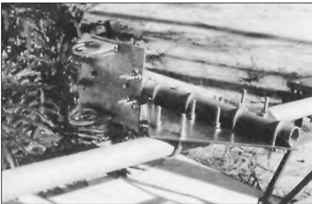
Fig 38—Close-up of the PVRC mount. The long pipe (horizontal in this photo) is the rotating mast. The U bolts in the vertical plate at the left are ready to accept the antenna boom. The heads of two locking pins (bolts) are visible at the midline of the boom plate. The other two pins help secure the horizontal pipe to the large steel mast plate. (The head of the bolt nearest the camera blends in with the right hand leg of the U bolt behind it.)
