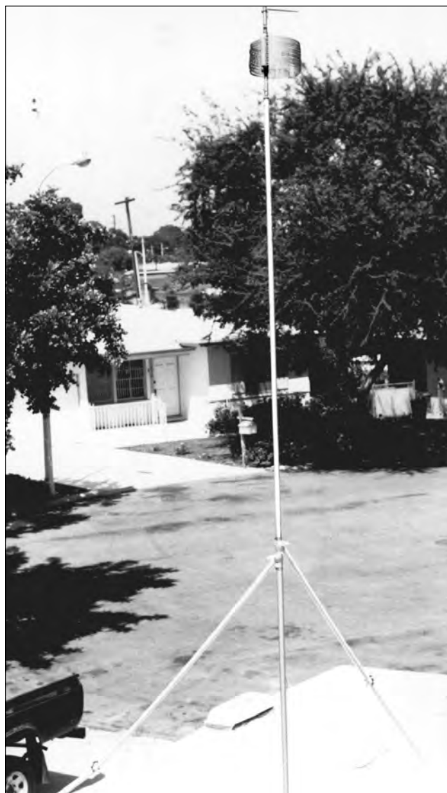
Fig 17 —Photo showing the two support bracket poles bracing the bottom section of the antenna. The top tuning whip is evident above the homemade loading coil at the top of the bottom section.
