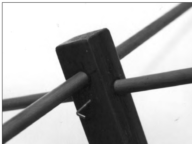
Fig 19—Photo of one end of the VE7CA quad with the two spreaders inserted.
