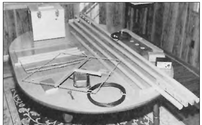
Fig 49—The complete portable quad, broken down for travel. Visible in the foreground is the driven element. The pine box in the background is a carrying case for equipment and accessories. A hole in the lid accepts the mast, so the box doubles as a base for a short mast during portable operation. (W1MPO photo)
